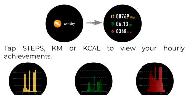
NOTE : Smartwatches use multi-axis inertial sensors called accelerometers. These detect wrist movement in order to measure steps. However, some wrist actions whilst standing or sitting can mimic the arm movement of a step and can therefore falsely record steps. The step count recorded each day should be used as a guide only.
